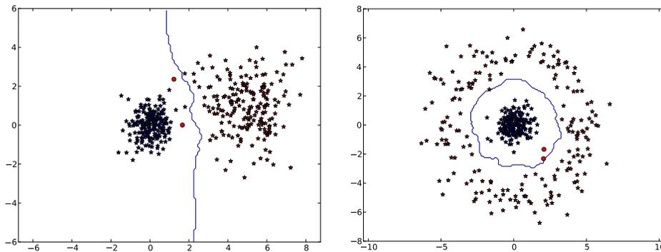
Figure 8.1: Classifying 2D data using a  $k$  nearest neighbor classifier. For each example the color shows the class label (blue and red). Correctly classified points are shown with stars and misclassified points with circles. The curve is the classifier decision boundary.
