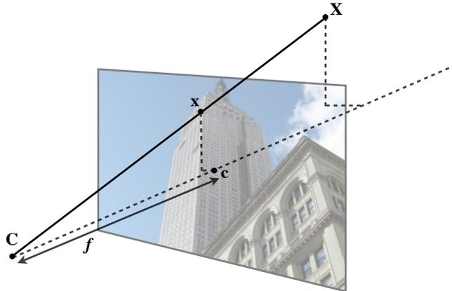
Figure 4.1: The pin-hole camera model. The image point  $x$  is at the intersection of the image plane and the line joining the 3D point  $X$  and the camera center  $C$ . The dashed line is the optical axis of the camera.
