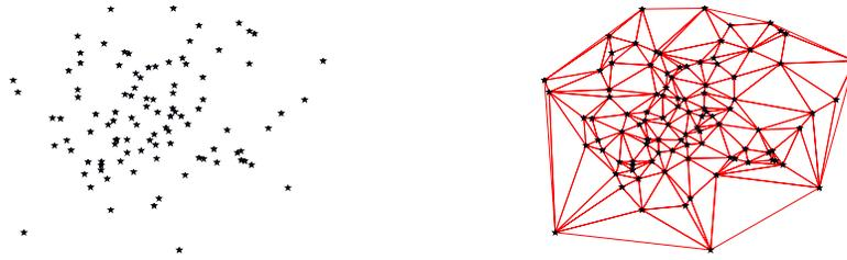
Figure 3.4: An example of Delaunay triangulation of a set of random 2D points.
